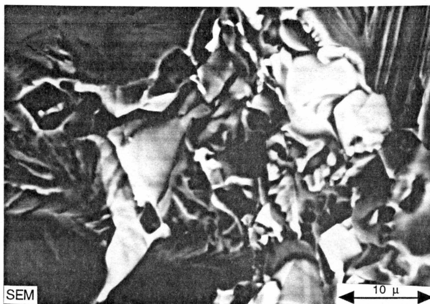
Figure 61. CN-7 : back-scatter electron image (BSE) of a sample annealed 12h at 1500°C and tested in tension at room temperature in air. Light-contrast phase is the \text{Cr}_2\text{Nb} intermetallic and the dark-contrast phase is the Cr-rich matrix.
