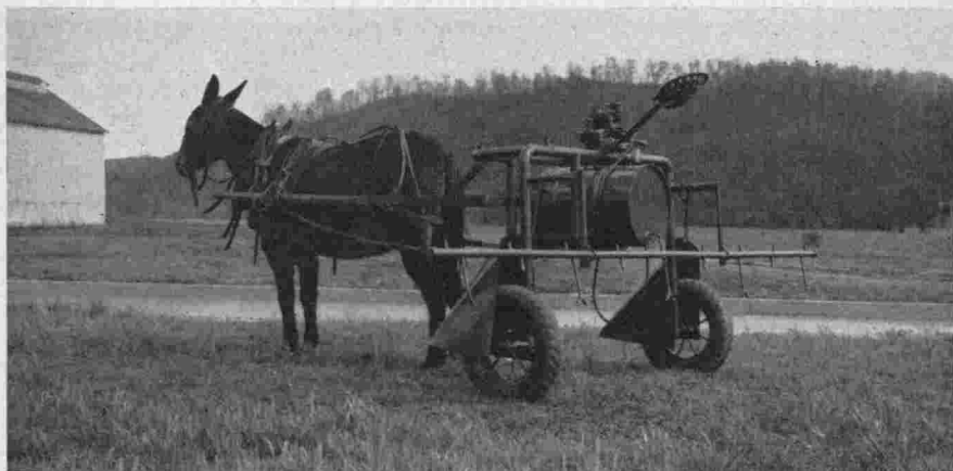
Figure 4—A high-clearance cotton sprayer developed at the Experiment Station.
