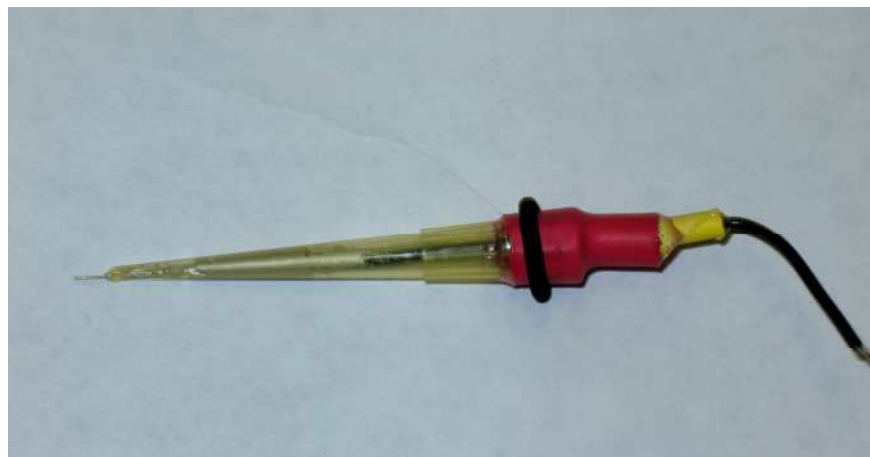
Figure 3.1. Disposable mercury-gold–microwire electrode with a 100 \mu\text{M} diameter gold wire inserted into a 200 \mu\text{L} disposable pipette tip.
