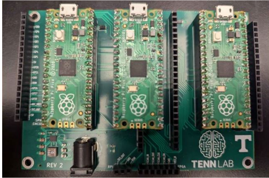
Figure 2.1: Neuromorphic Kit with Three Raspberry Pi Picos
