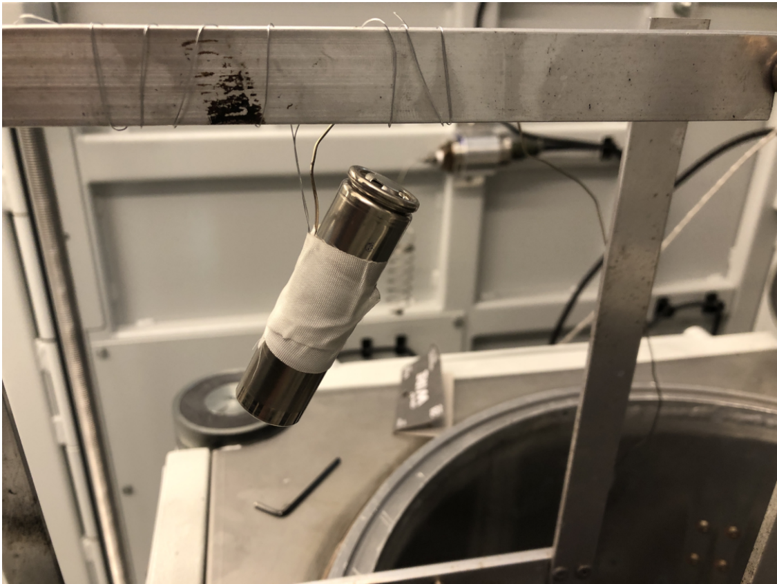
Figure 4.4: Molicel 18650 set up for a thermal runaway test.
