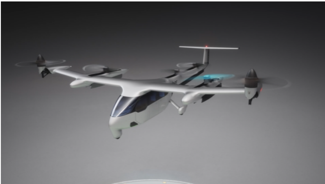
Figure 1.1: Uber Elevate rendering of a potential eVTOL design [12].
