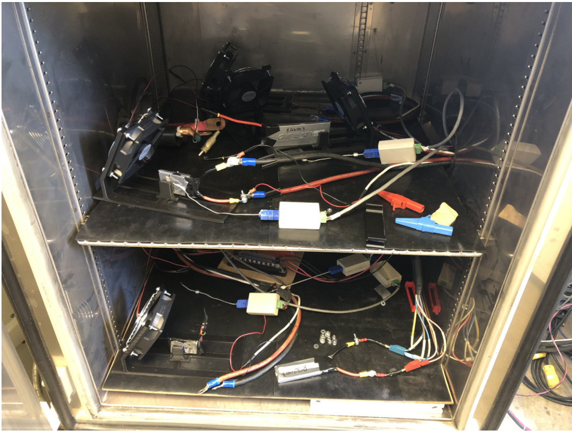
Figure 2.3: Setup for the endurance tests inside of the environmental chamber.
