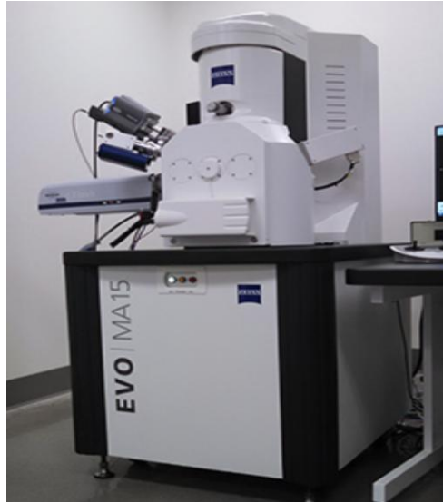
Figure 3.3: Zeiss EVO SEM with integrated EDS.
