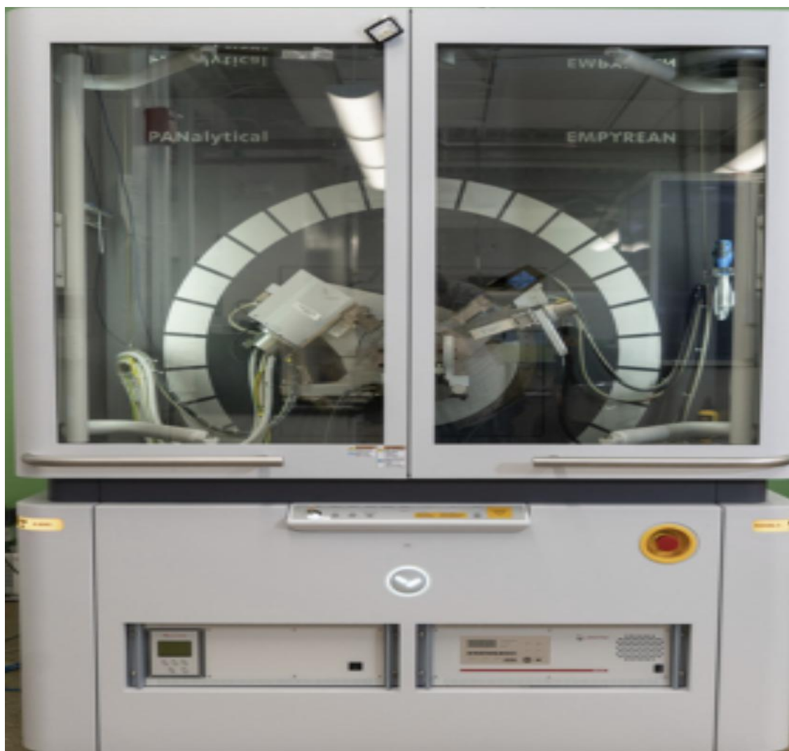
Figure 3.2: PANalytical EMPYREAN XRD instrument setup.
