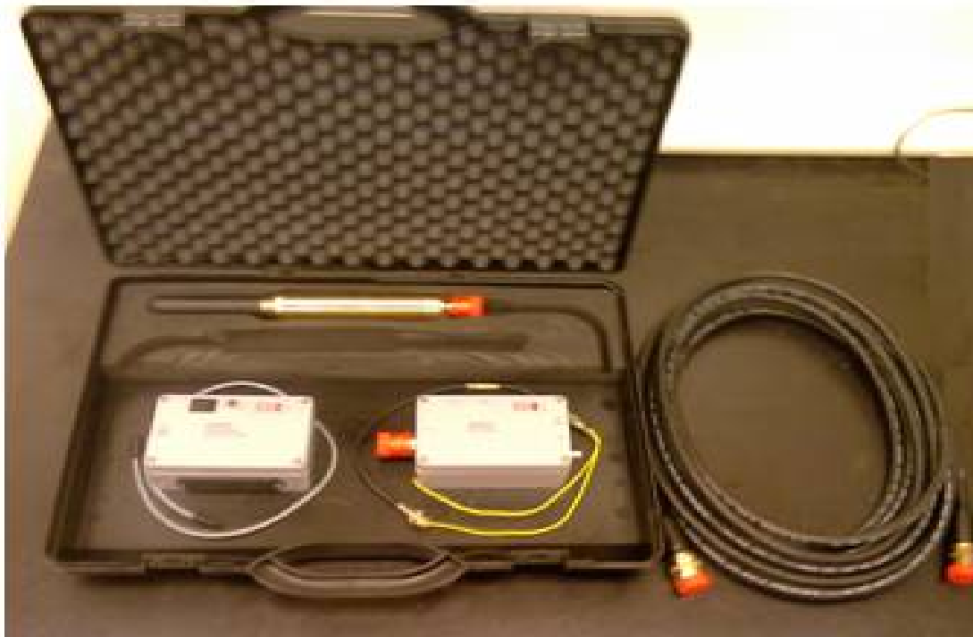
Figure 4.8.1: RESON TC 4032 hydrophone with cable, input module (right), and DC power supply (left); approximate length is 30cm.
