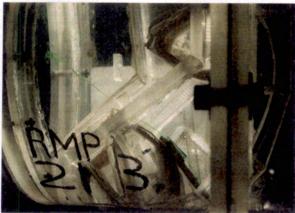
b. Zone 3, Ramp Displaced Toward Sidewall
