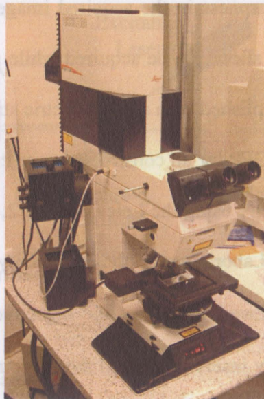
Figure 5.4. Leica TCS SP2 laser confocal microscope.
