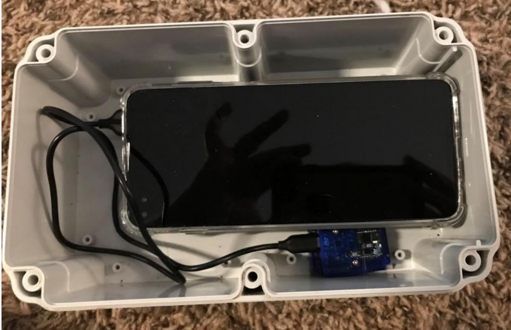
Figure 7. Secured sensor and phone within NEMA Enclosure.
