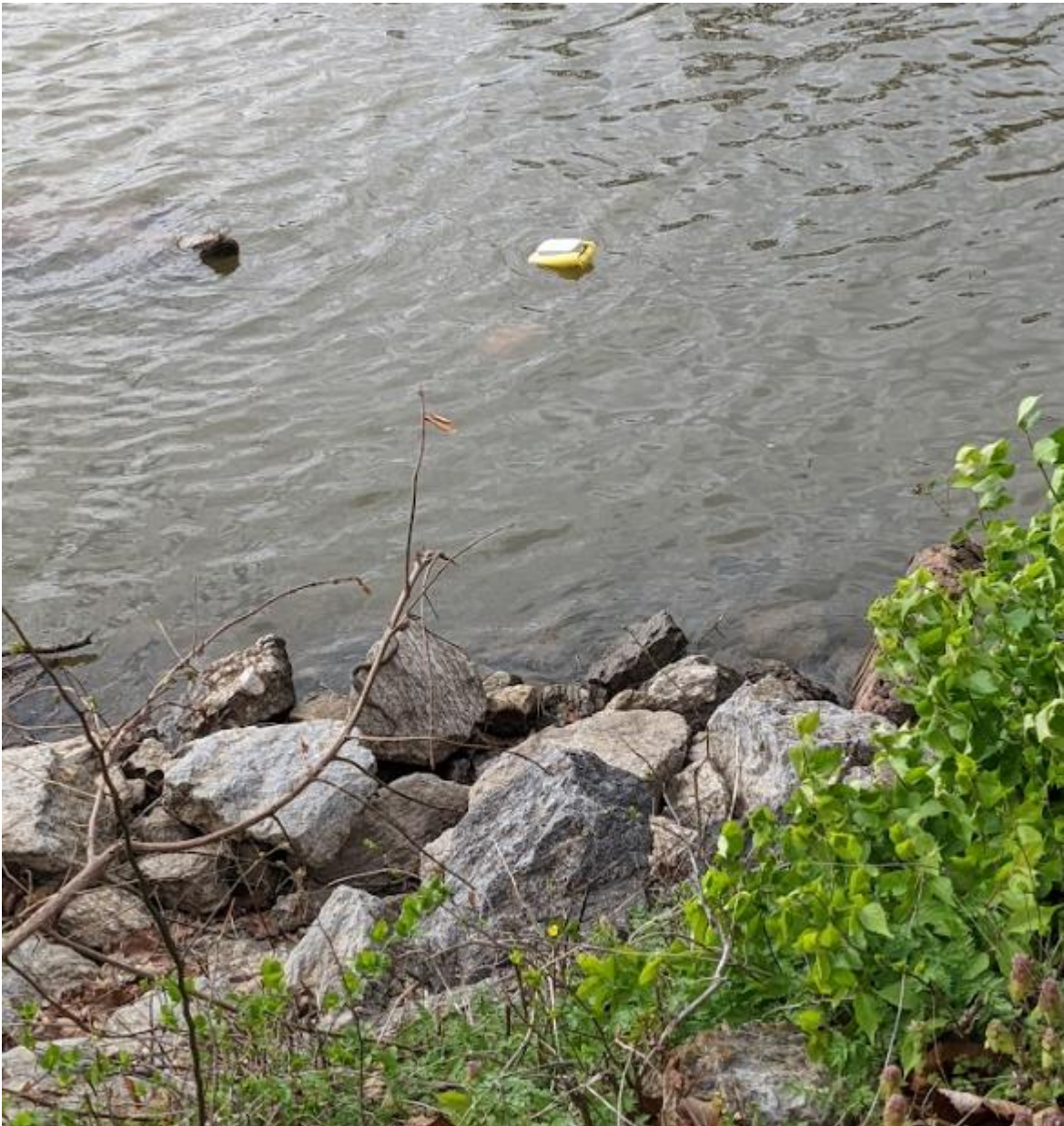
Figure 9. Floating buoy with phone inside tracking submerged manikin.
