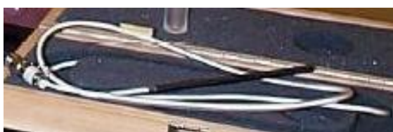
Figure 11: A thimble ionization chamber commonly used in radiation therapy quality assurance testing.
