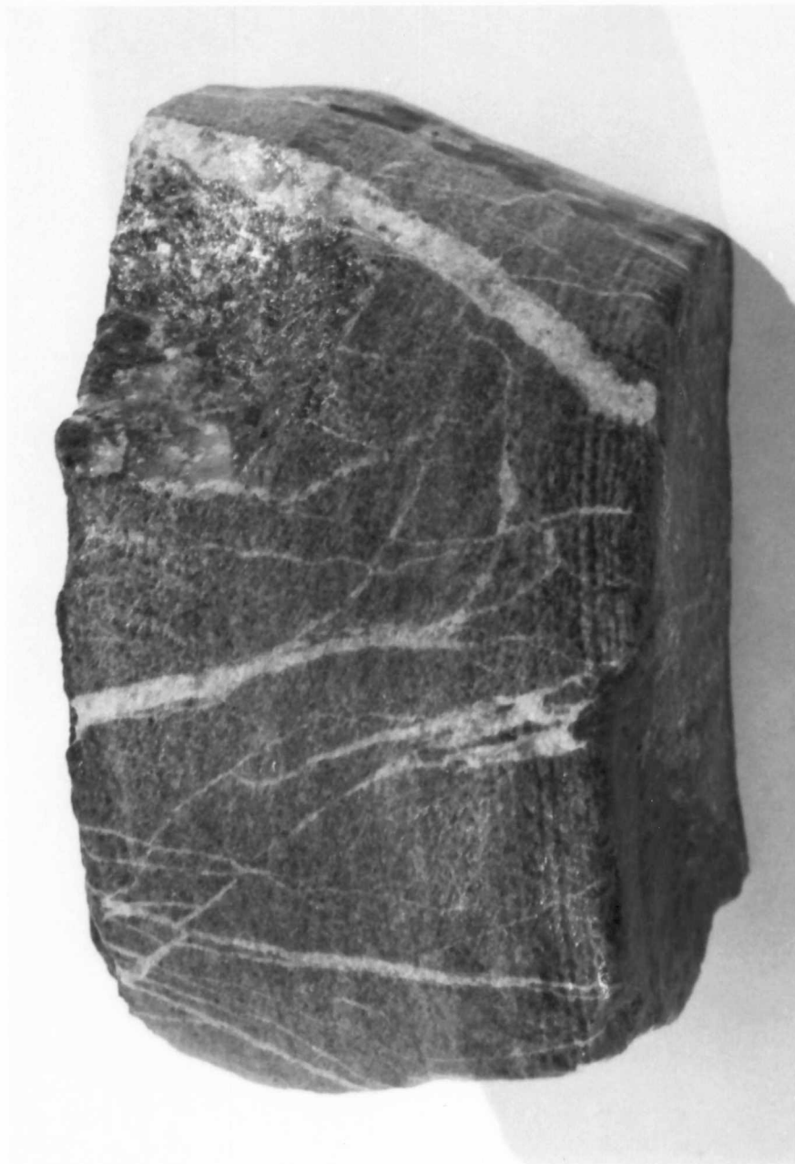
Figure 5. Photograph of drill core in the Southern Conasauga Belt taken at a depth of 23 m. This core (approximately 3.5 cm across) displays abundant jointing in a siltstone bed.
