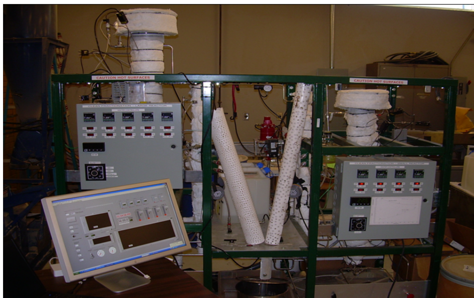
Figure 13. Organosolv fractionation reactor with computer interface.
