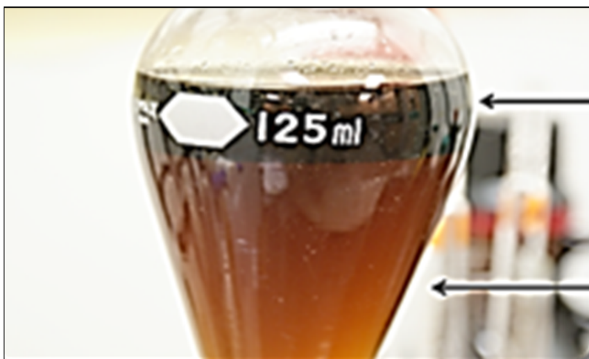
Figure 16. Phase separation between organic (top) and aqueous layer (bottom).
