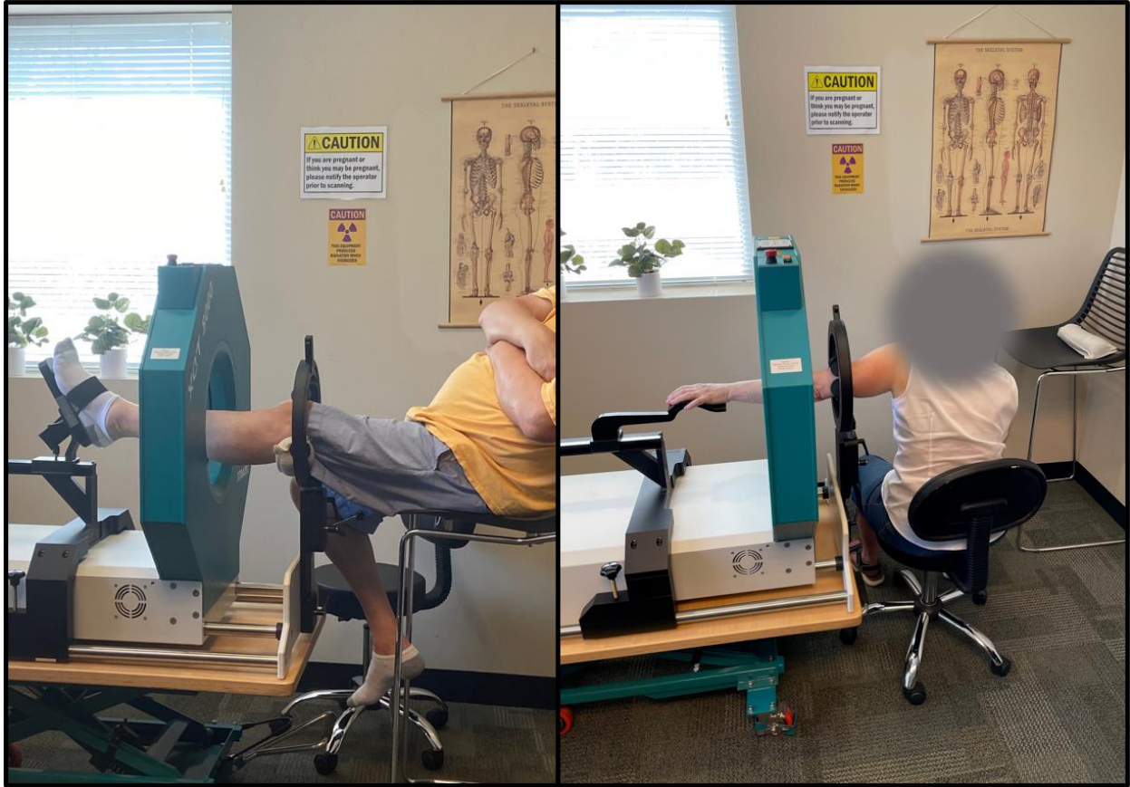
Figure 1.1. Positioning of participants in pQCT scanner. Left: Participant is seated with non-dominant leg in scanner with no visible leg rotation and foot vertical. Right: Participants non-dominant arm is abducted roughly 90 degrees with forearm pronated.
