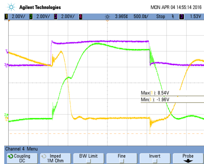
Figure 4.37 Experimental Switching Waveforms driving 133nF Gate Capacitance
