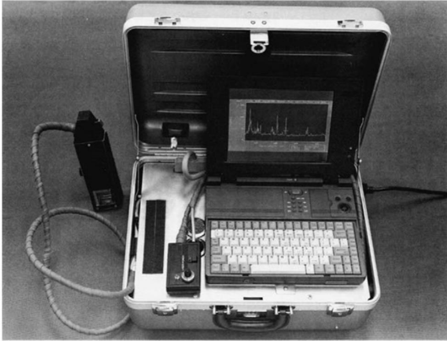
Figure 2.3 (above): Example of portable LIBS system developed by Yamamoto et al. [38].
