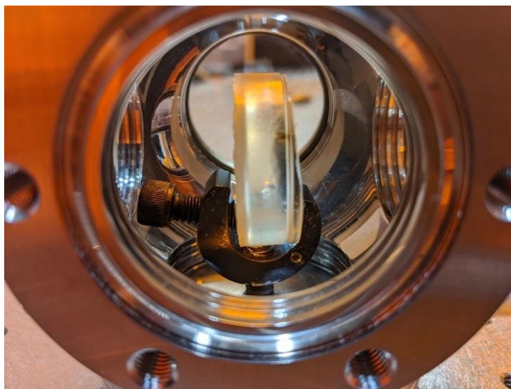
Figure 3.13 (above): Modification of sample chamber to allow mounting of solid samples
