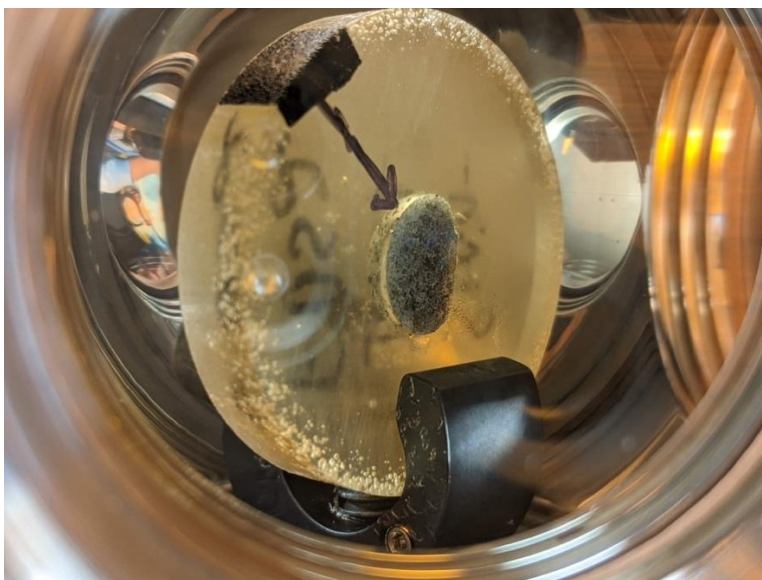
Figure 3.23 (above): Non-radioactive nuclear melt glass sample used in the fs-LIBS experiments
