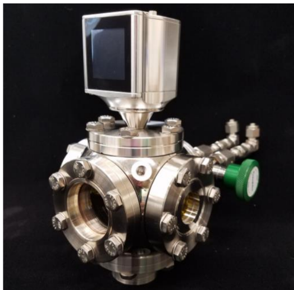
Figure 2.6 (above): Chamber designed by Martin et al. to assay \text{UF}_6 for LISA-UE project [47].
