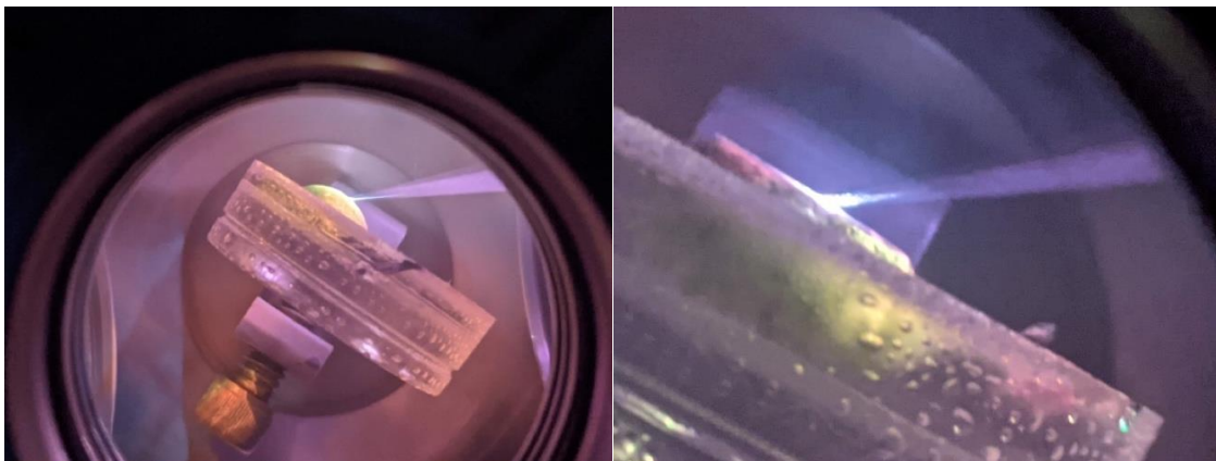
Figure 3.32 (left) & 3.33 (right): fs-LIBS of radioactive nuclear melt glass
