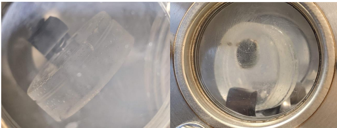
Figure 3.37 (left) & 3.38 (right): Smeared sapphire windows in the sample chamber as a result of the initial decontamination procedure that used “RadiacWash” to safely clean the sample chambers.
