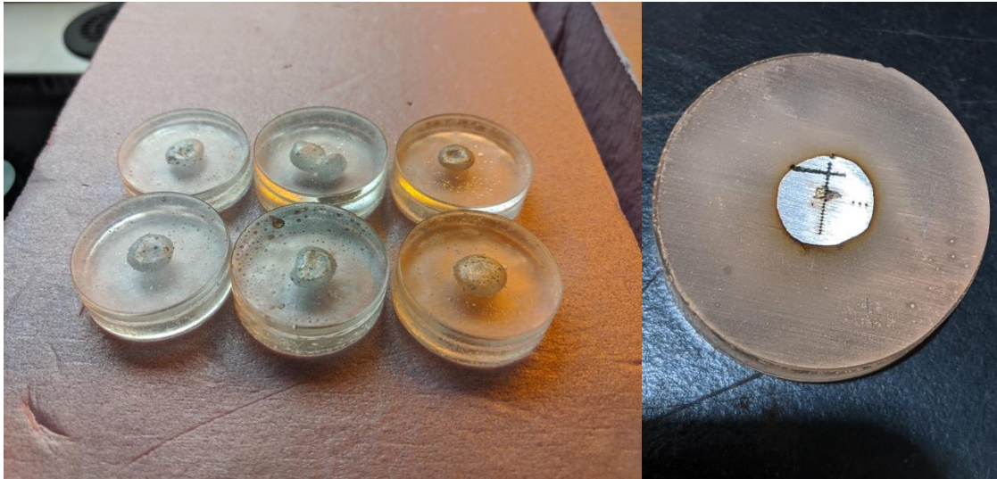
Figure 3.15 (left) & 3.16 (right): Un-sanded Aluminum samples appear on the left while one of the sanded samples is shown in the photo on the right.
