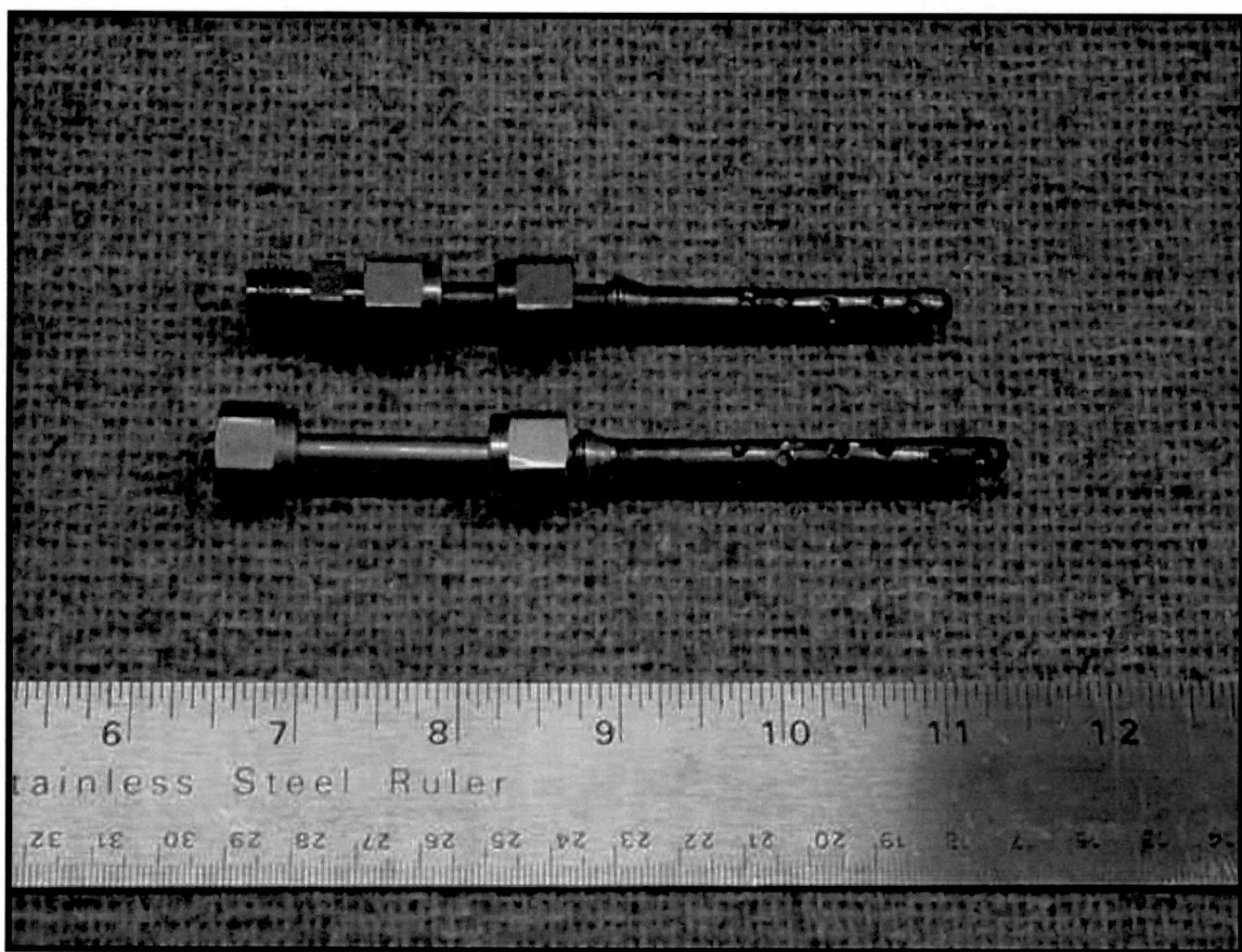
Figure 3.4 – Sample probes for smoke measurement.
