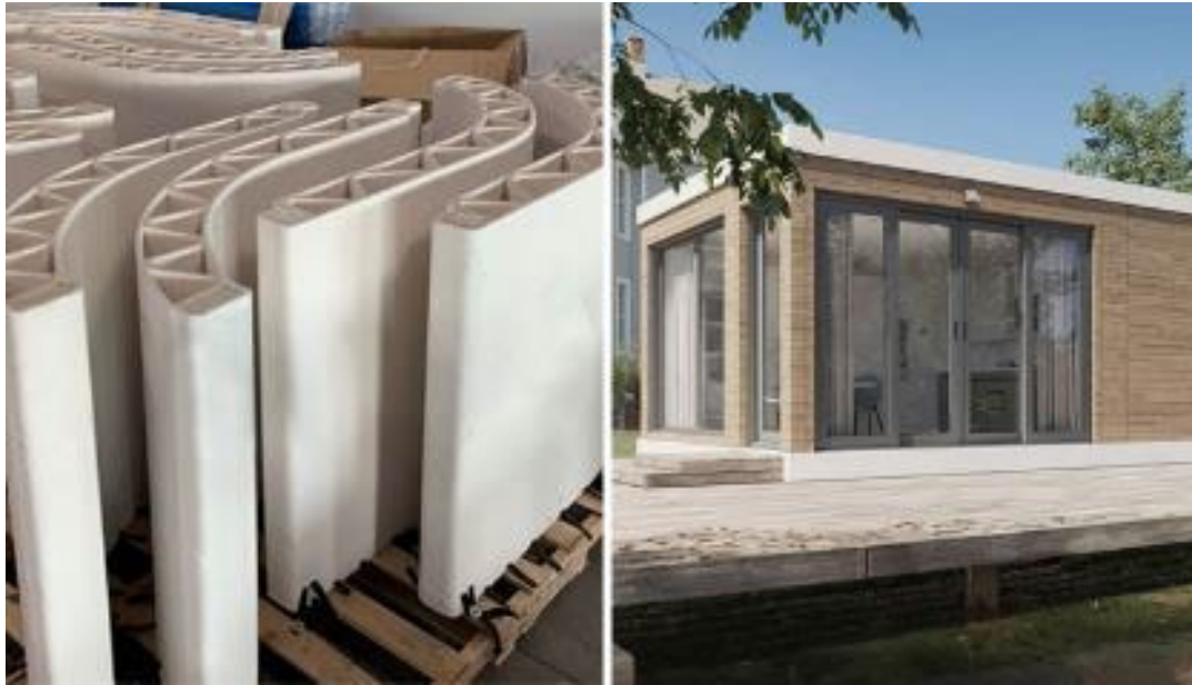
Figure 3 Photopolymers are emerging as a polymer feedstock for LFAM, with applications such as this 3D printed 350 sq. ft. building. Note the use of limited infill and thick beads, as in other LFAM methods (Source: Mighty Buildings [8]).
