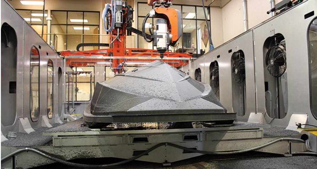
Figure 2 Large-scale thermoplastic AM is focused primarily on the tooling industry. Materials such as carbon fiber-filled ABS are used in marine applications such as this boat hull mold, which was printed on a Thermwood Large Scale Additive Manufacturing (LSAM) system with a 10' x 20' work table (Source: Composites World[16]).
