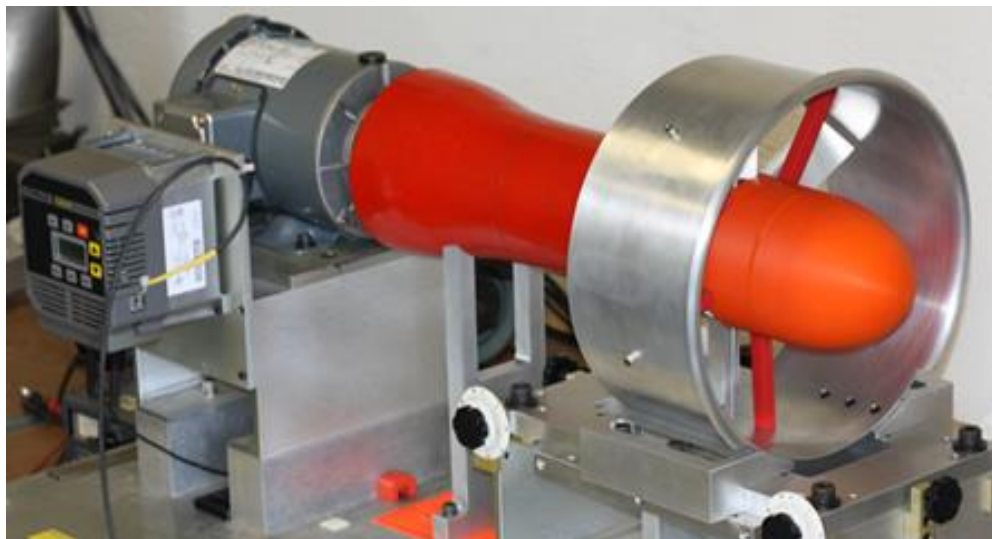
Figure 19 – Experimental Fan Rig with 3-D Printed Components.
