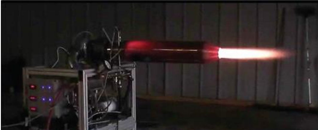
Figure 18 – GTE J1-H-01 Operating in Full Augmentation.
