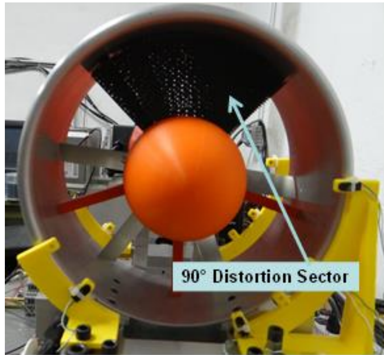
Figure 22 – 90° Inlet Distortion Sector Installed in Fan Rig.
