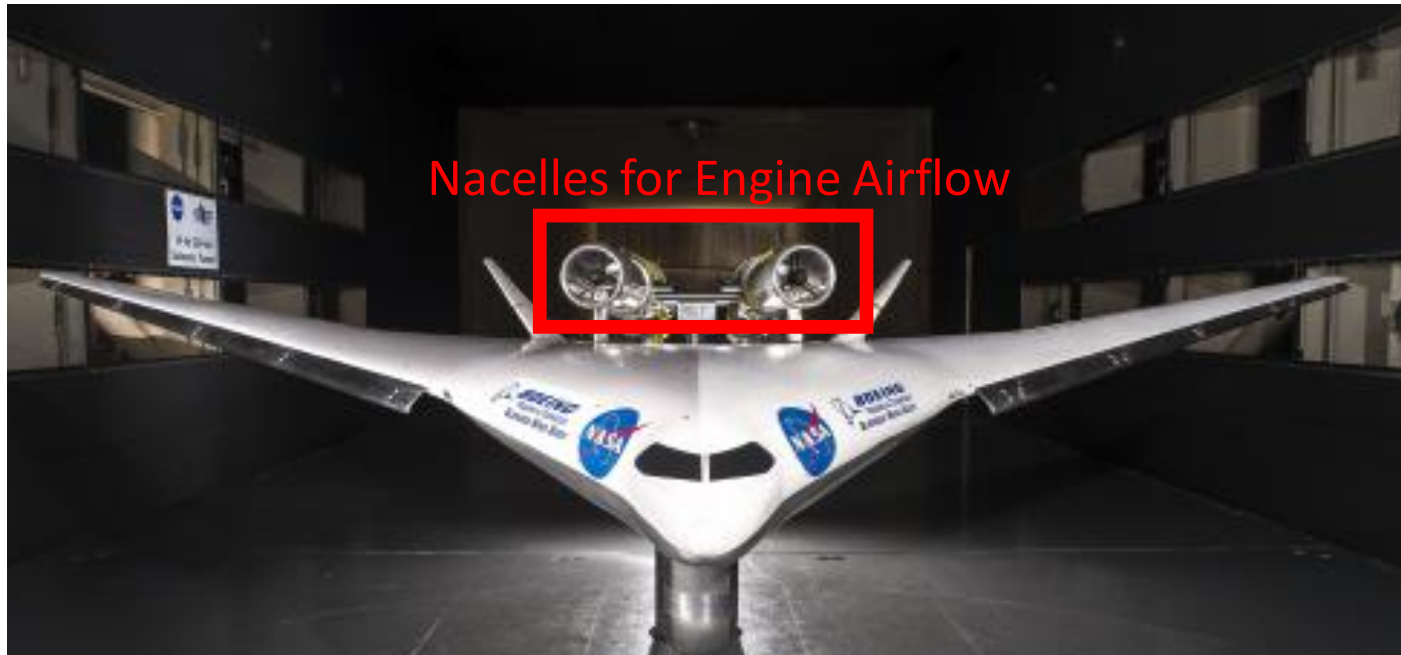
Figure 1 – Wind Tunnel Test of NASA Hybrid Wind Body (HWB) Model 1 .
