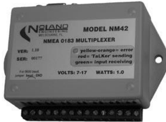
Figure 10: The NMEA 0183 multiplexer used to combine the two distance sensors, depth data and GPS data into a single data string ( http://nolandeng.com/nm42.php , accessed January 2012).
