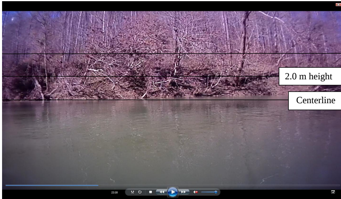
Figure 6: Photo from New River (TN) showing: Bank Angle = 2.45, Bank Height = 4.5 ft, Surface Protection = 2.45, Riparian Diversity = 2.45.
