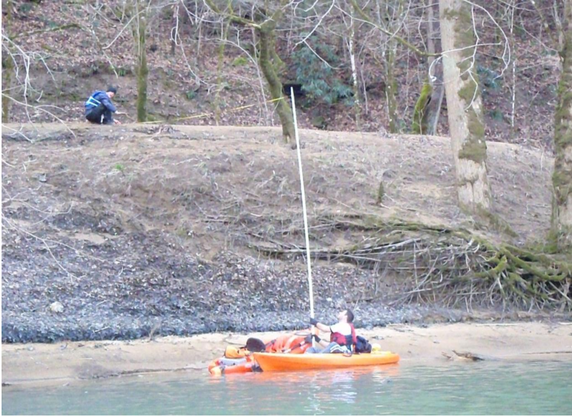
Figure 29: New River (TN) Bank Height Field Measurement.
