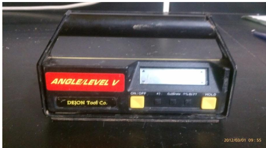
Figure 26: Inclinometer used to take bank angle measurements in the field.
