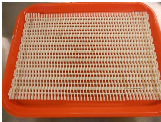
Figure I-0-5 Mesh conveyor belt
