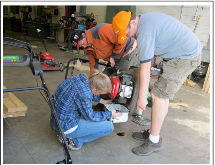
Joe Yantis , Chanci King and Grant Davis drain the oil out of one of the mowers.
