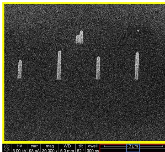
Figure 20. An initial video frame highlighted with the segmented parts – yellow is the image, red the scalebar and blue the scale.
