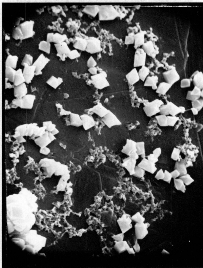
Figure 4-1. SEM micrograph for \text{Ca(OH)}_2 from hot lime slaked in laboratory, 5000 X, magnification.
