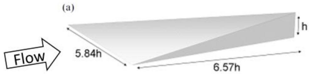
Figure 2.5. Optimized dimensions of a VG in supersonic flow [43]
