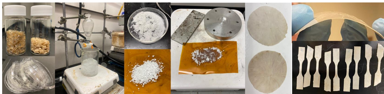
Figure 6: Images showing the depolymerized and virgin PET, the precipitation in methanol setup, the blended material, the melting setup on the hot plate, the melted virgin PET sheets, and virgin PET dog bones.
