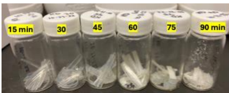
Figure 15: The change in flake appearance and structure with depolymerization time from 15 to 90 minutes reacted.
