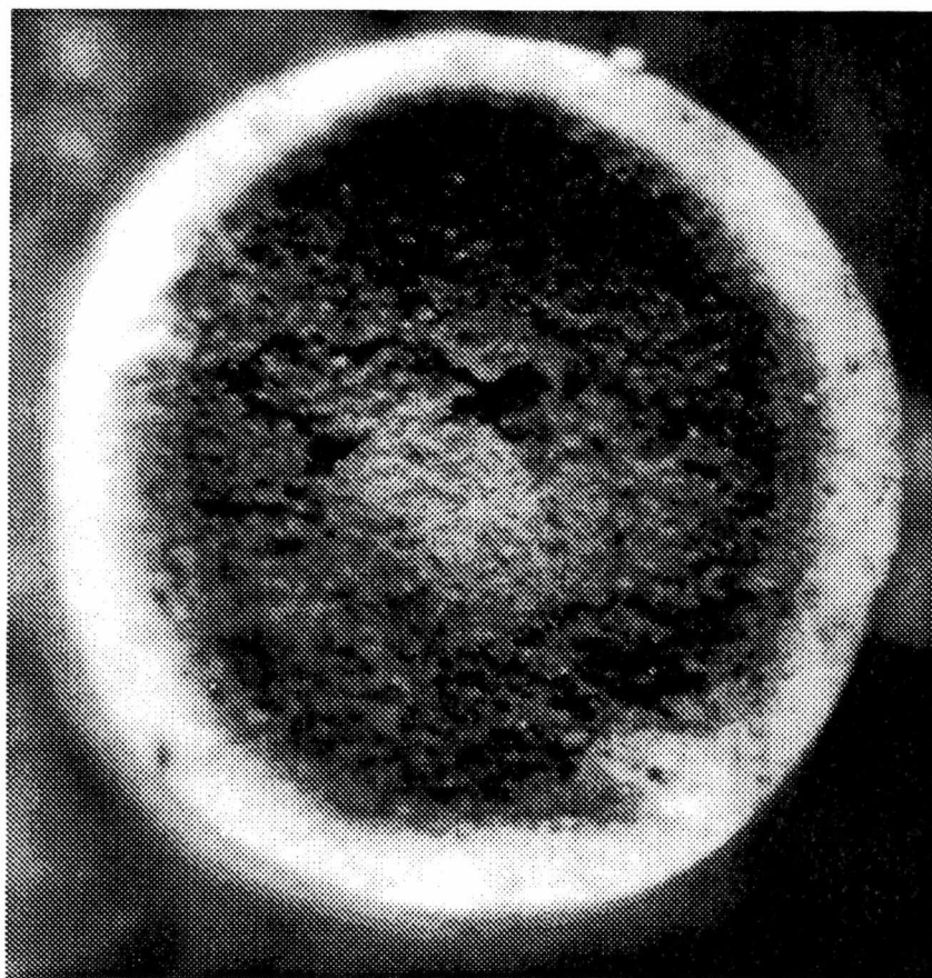
Figure 4.11. Optical image of 1/16-in. AgZ from bed with an average conversion of ~19% (ORNL PHOTO 5085-94).
