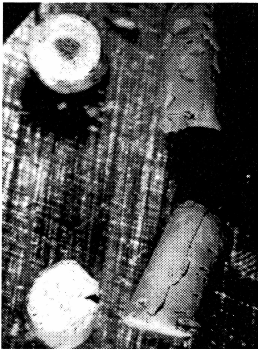
Figure 4.12. Optical image of 1/16-in. AgZ from bed with an average conversion of ~40% (ORNL PHOTO 5084-94).
