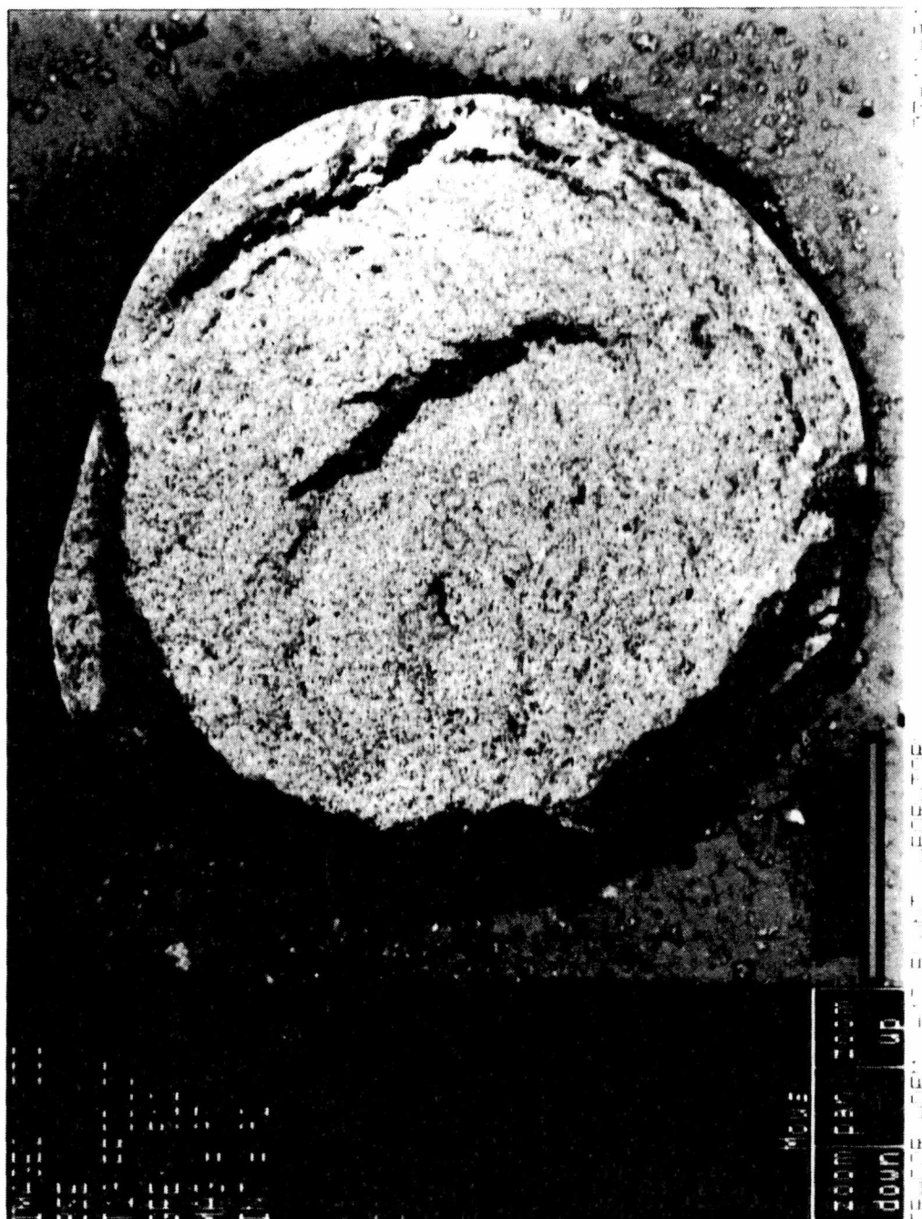
Figure 4.1. Back-scattered electron image of Test 19 1/16-in. AgZ showing uniform silver distribution.
