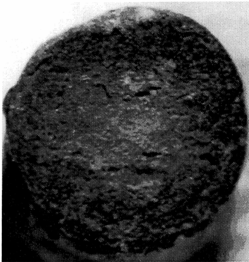
Figure 4.10. Optical image of 1/16-in. AgZ from bed with an average conversion of ~3% (ORNL PHOTO 5081-94).
