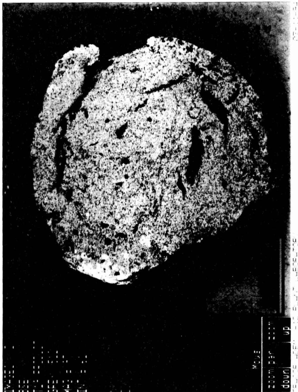
Figure 4.2. Back-scattered electron image of Test 19 1/16-in. AgZ showing slightly nonuniform silver distribution.
