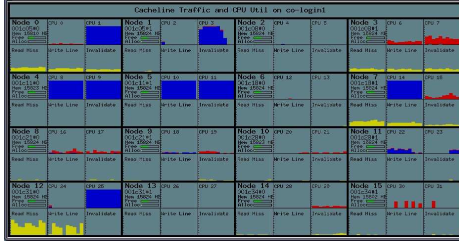
Figure 4.1: A screen shot of the performance monitoring tool pmsub on SGI Altix. The light yellow area reflects how many remote memory accesses have occurred.
