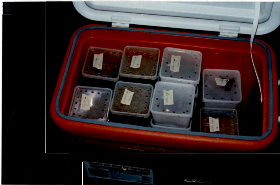
Figure 6. The Ice Chests Used as Conditioning Chambers to Obtain Initial Moisture Conditions for All Tests.
