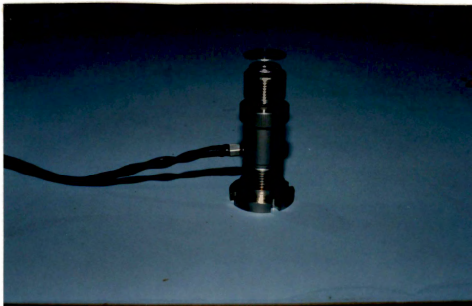
Figure 4. 10-g Load Cell Used to Measure the Progressive Weight Gain of the Burley Tobacco Leaves in the Absorption Tests.
