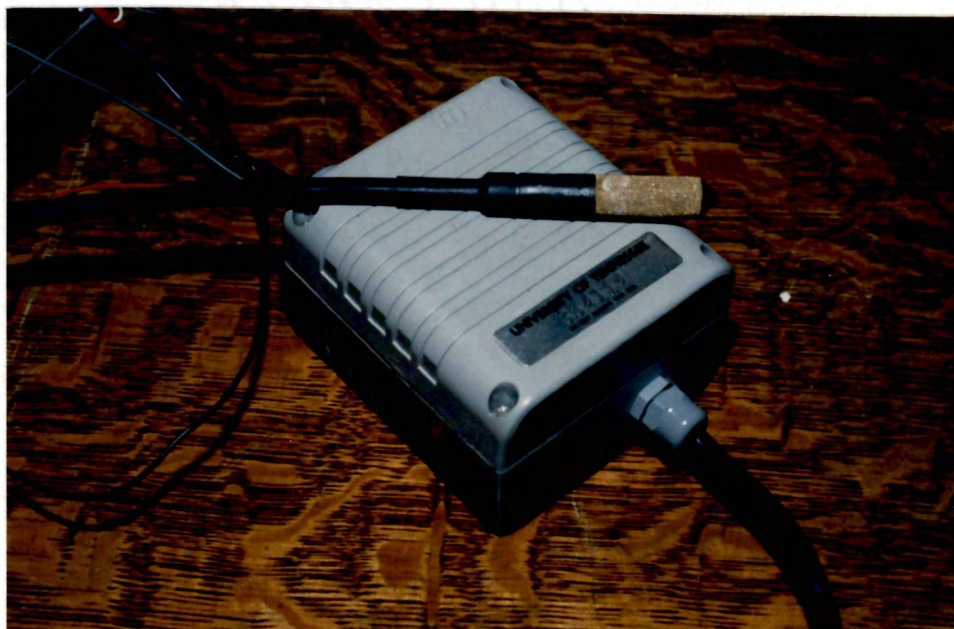
Figure 5. Probe Used to Measure the Relative Humidity Within the Environmental Chamber for the Absorption Tests of Burley Tobacco Leaves.
