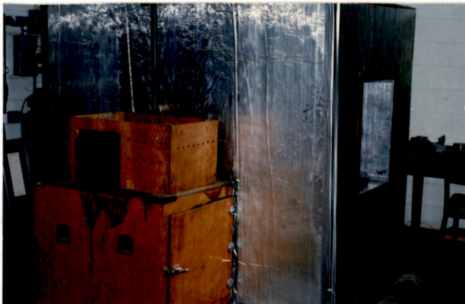
Figure 3. Air Conditioned Chamber Over the Leaf and Salt Chambers Used for the Absorption Tests of Burley Tobacco Leaves.
