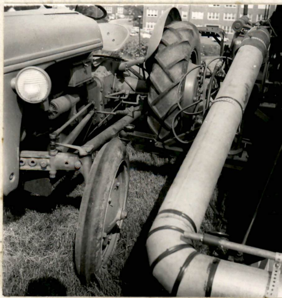
Figure 14. Front View of Combine, Side Mounted on Tractor, Showing Tractor Support Frame, Combine Ball and Socket Hitch
