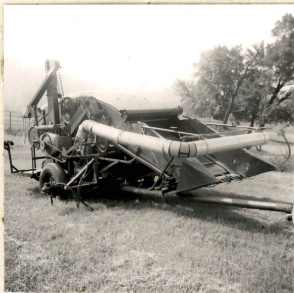
Figure 12. Three-Quarter Right Front View of Combine Showing Blower and Duct System for Air Blast Wind Reel
