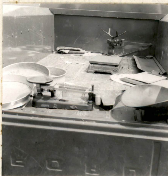
Figure 18. Hand Sieves, Balance Scales, and Trays For Preparation and Measurement of Combine Seed Samples
