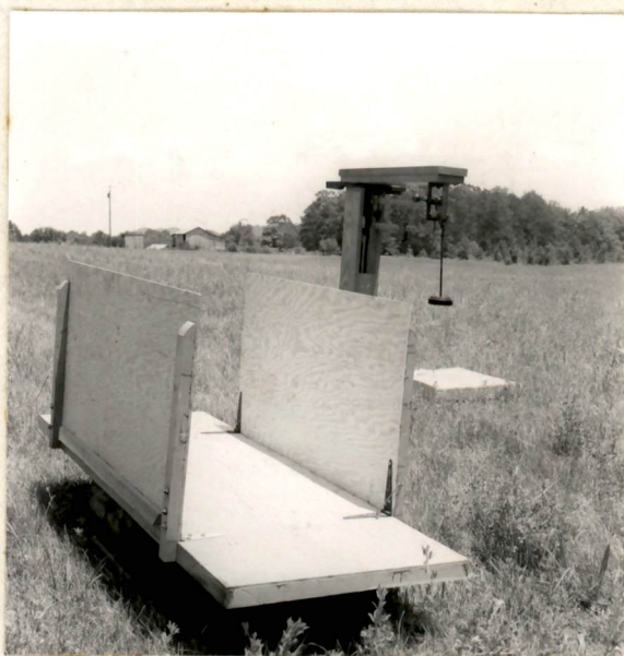
Figure 17. Platform Scale with Special Extension to Weigh Combine Rack and Shoe Discharge Material
