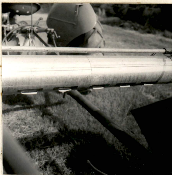
Figure 13. Plenum Duct of Air Blast Wind Reel With Slotted Orifices
