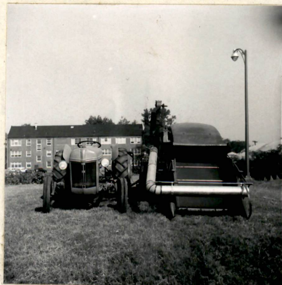
Figure 1. Front View of Allis Chalmers Model 40 Combine Side Mounted on Ford-Ferguson Model 9N Tractor
