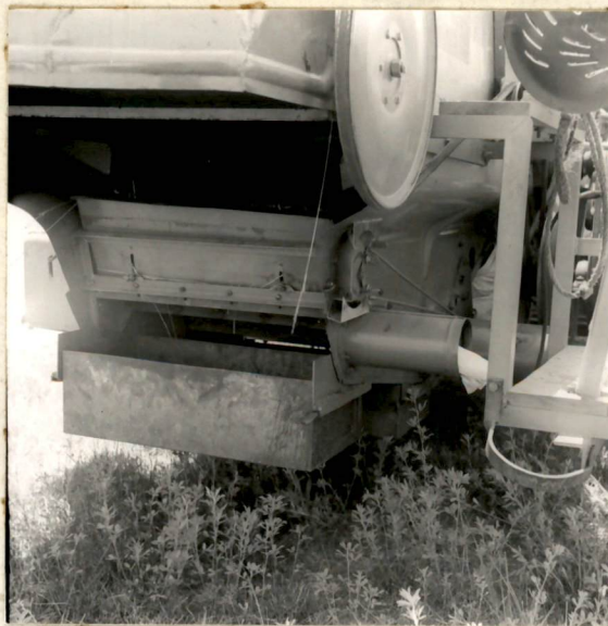
Figure 7. Sliding Trays Under Grain Bin Auger and Tailing Auger, For Collection of Seed Samples
