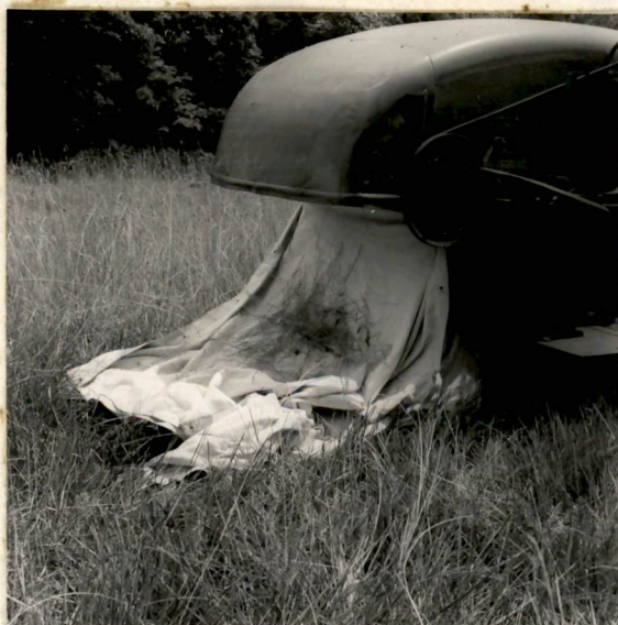
Figure 9. Canvas Sheets Attached to Rear of Combine to Collect Discharged Material
