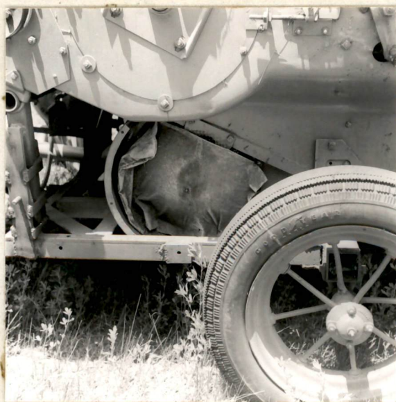
Figure 19. Left Side View of Combine Showing Cloth Cover on Blower Intake Screen
