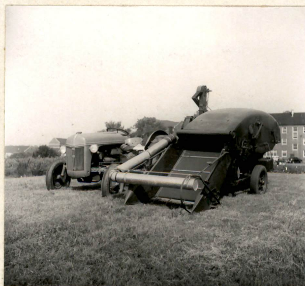
Figure 2. Three-Quarter Front View of Experimental Combine, Side Mounted on Tractor
