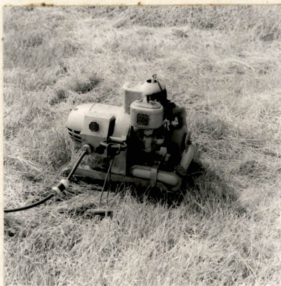
Figure 16. Gasoline Engine, Electric Generator Used to Provide Power for Seed Cleaner
