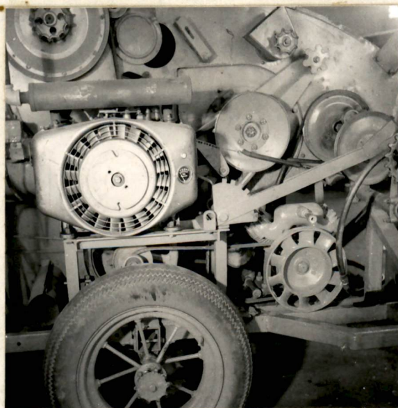
Figure 3. Right Side View of Combine Showing Location of Onan Engine
