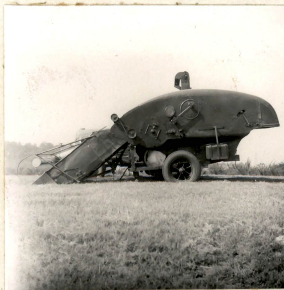
Figure 4. Left Side View of Combine Showing Location of Gas Tank
