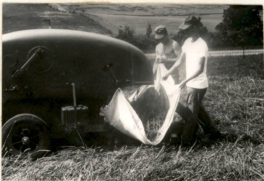
Figure 10. Field Operation of Combine Showing Collection of Combine Rack and Shoe Discharge on Canvas Sheets
