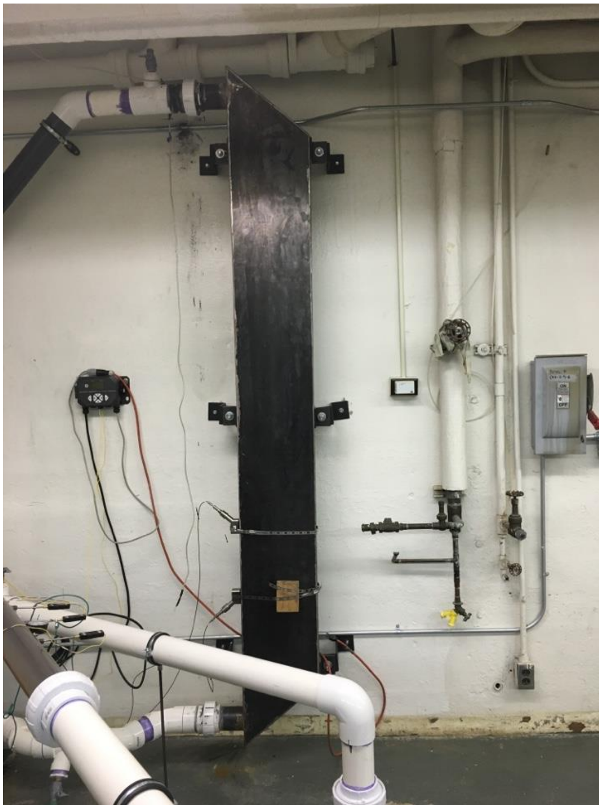
Figure 15: Picture of the steel test section of the flow loop, meant to simulate downcomer of an integral reactor
