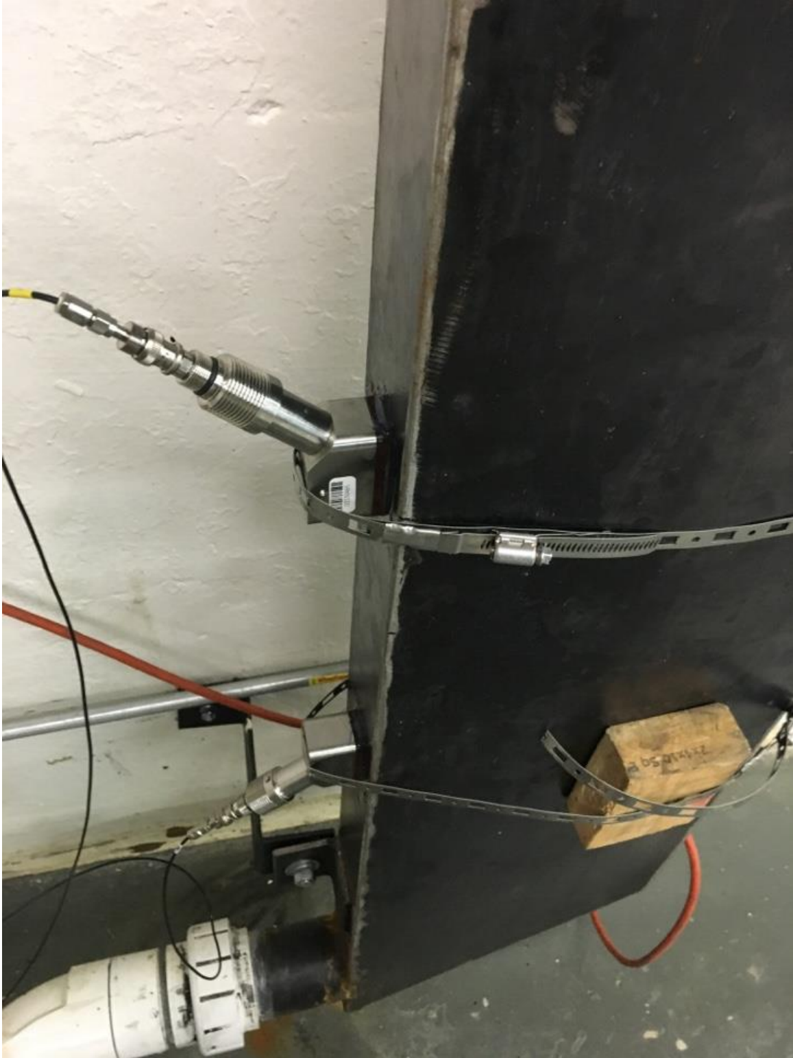
Figure 20: Picture of ultrasonic transducers mounted on test section. Coupling grease is placed between transducers and steel.
