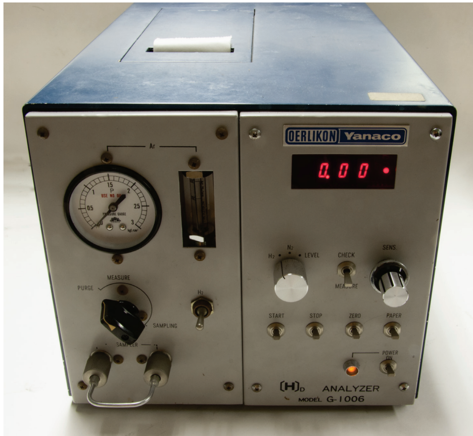
Figure 30. Oerlikon-Yanaco Hydrogen Analyzer for Hydrogen Measurement.
