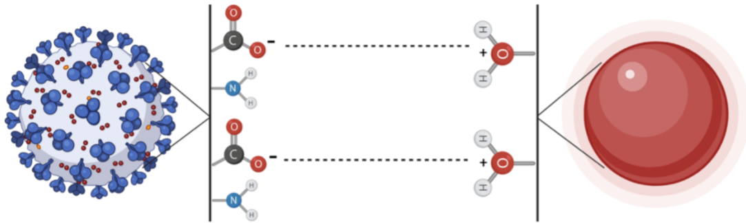
Figure 2.3 Schematic of electrostatic attraction between a viral particle (left) and iron oxide-coated sand (right) through negatively charged carboxyl (-COO - ) and positively charged hydroxyl (-OH 2 + ) groups [Created with BioRender].
