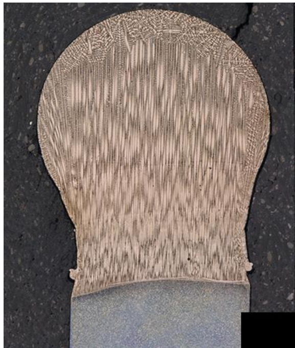
Figure 67: Change in deposit width from less than the width of the original substrate to greater than the original substrate width at higher layer numbers results in off-axis columnar growth. Off-axis growth occurs only at locations where the deposit width exceeds the substrate width.
