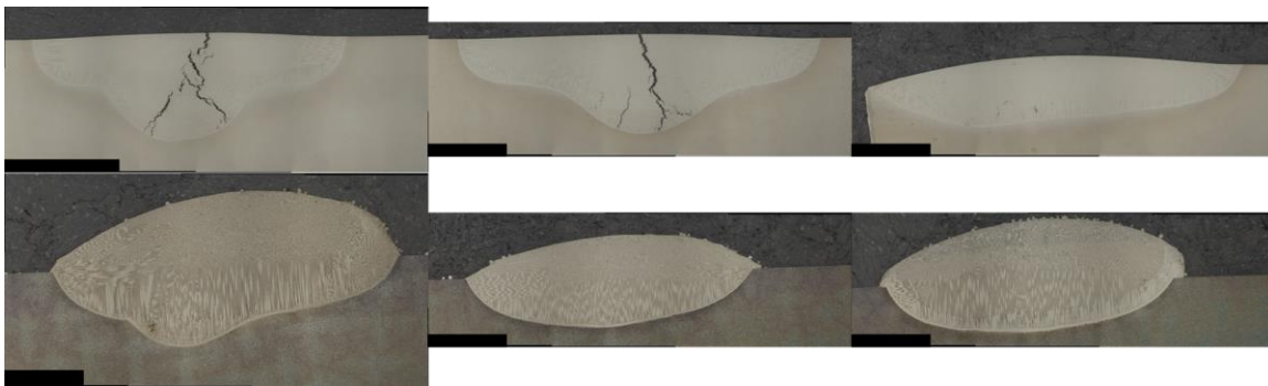
Figure 79: Spiral Sample D-1 through D-3 track geometry without mass addition (top) and Sample H-1 through H-3 track geometry without mass addition (bottom) transverse cross sections from 180-degree section location. Travel speed increasing from left to right.
