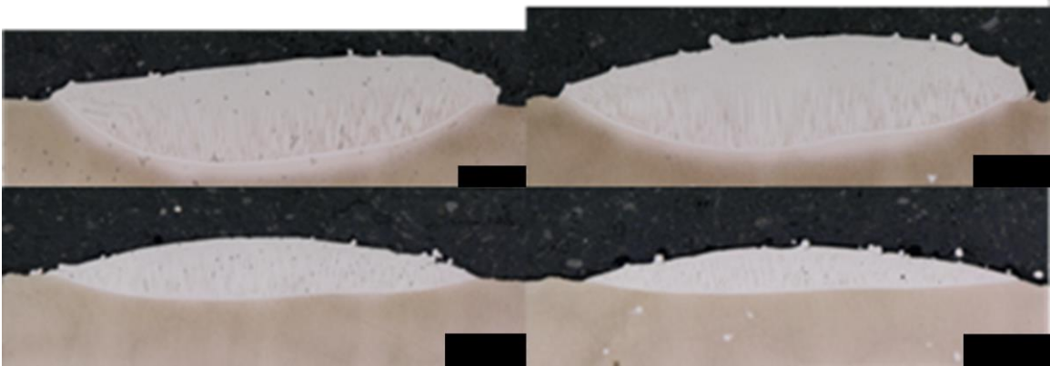
Figure 82: Sample J-1 (top left), J-2 (top right), J-3 (bottom left) and J-4 (bottom right) optical microscopy transverse cross sections for single-track thick plate deposits.
