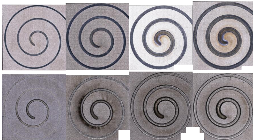
Figure 27: XY stitched optical images of deposits with without (top) and with (bottom) mass addition. Increasing laser power from left to right.
