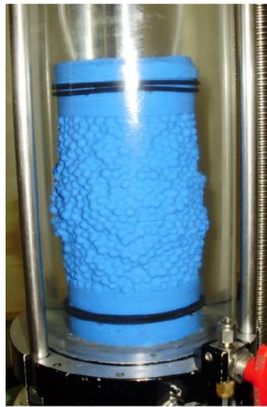
Figure 9.2. Experiment and DEM triaxial specimens (a) after isotropic compression and (b) after the shearing stage.
