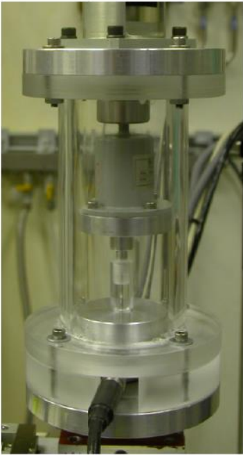
Figure 3.2. Photo and schematic of 1D compression test cell.
