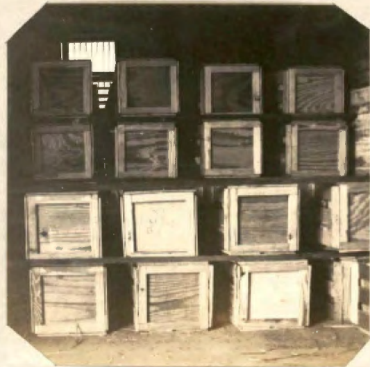
Crates properly stripped and packed in a ventilator car. This method of packing allows free circulation of air and still prevents excessive breakage in transit.
