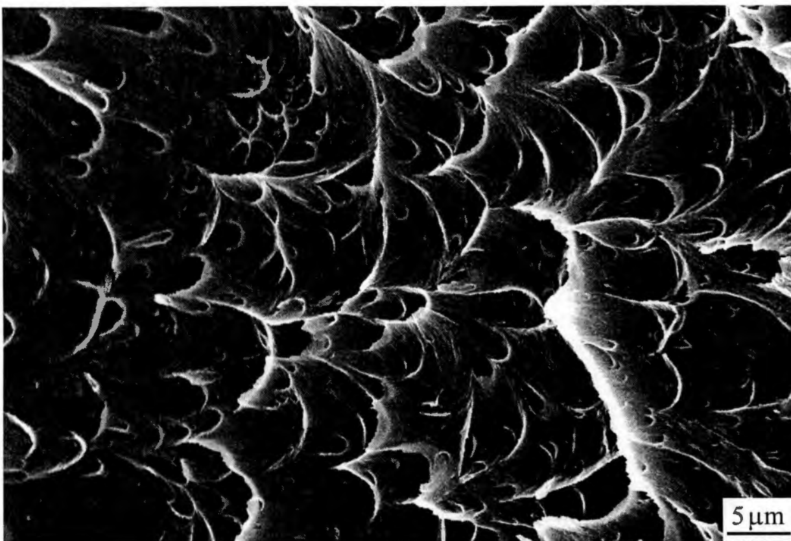
Figure 4.42. SEM micrograph of non-etched fracture surface of sPS50PPO blend melt crystallized at 220°C showing intraspherulitic fracture.
