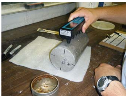
Figure 3: Surface Resistivity (SR) Testing Apparatus
