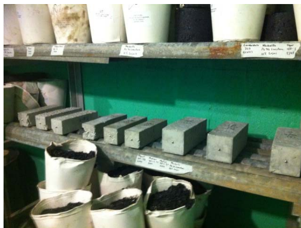
Figure 7: Storage of Shrinkage Prisms in Controlled Humidity Room
