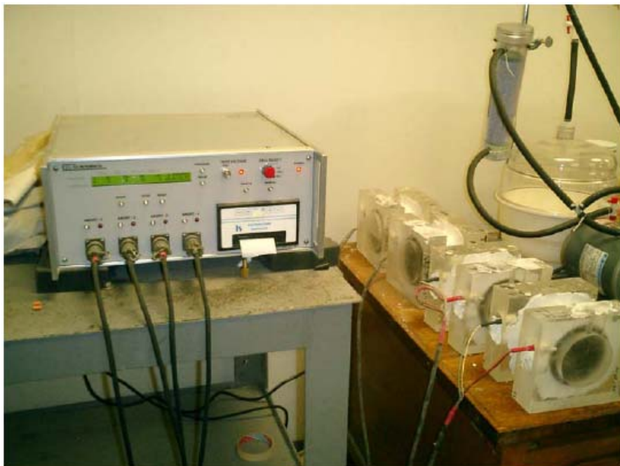
Figure 1: Rapid Chloride Ion Penetration (RCP) Testing Apparatus
