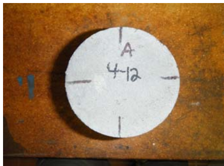
Figure 2: Top Surface Markings for SR test
