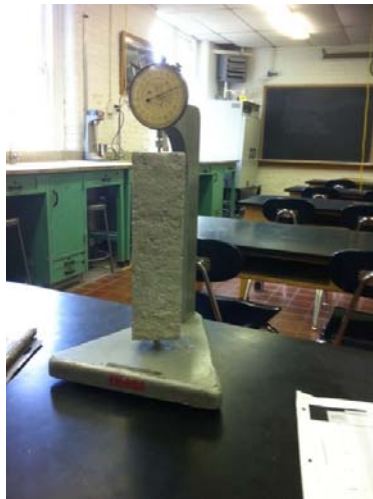
Figure 8: Length Comparator for Shrinkage Testing
