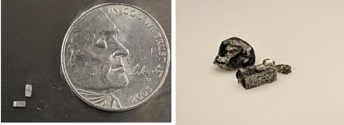
Figure 4-17. Representative melt wires prior to the test (left) and after the test (right).
