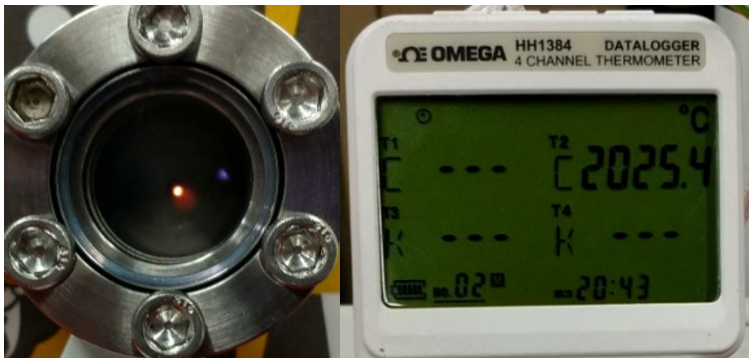
Figure 4-5. Specimen region viewed through the viewport (left) and thermocouple reader display (right) for the PPPT1 experiment.
