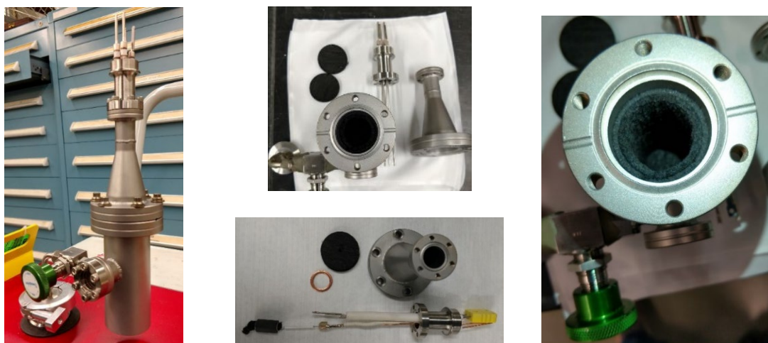
Figure 4-1. OUTSET attached to the Adixen ASM340d leak detector (left), component layout (top and bottom center), and view of the internal plenum (right).
