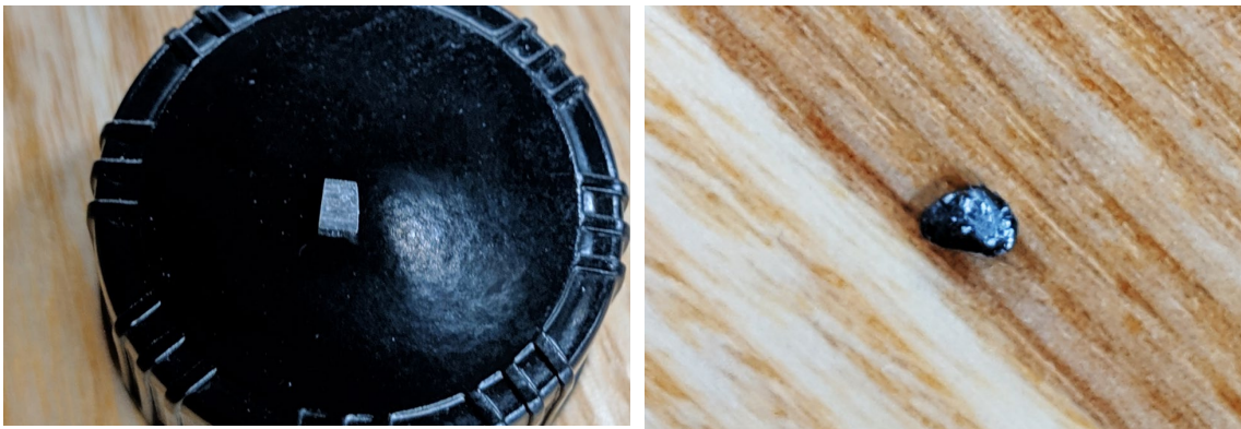
Figure 4-18. Melt wire prior to the test (left) and after the test (right).
