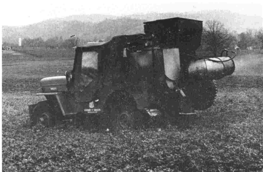
Figure 6. A jeep equipped with buffalo turbine for air blast and a mini-spin nozzle for low-volume application. It can apply as little as 8 ounces per acre.
