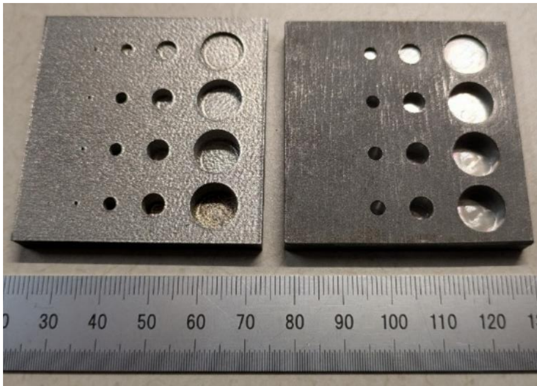
Figure 3.4. As-printed FBH1 sample (left) and as-machined FBH2 sample (right).
