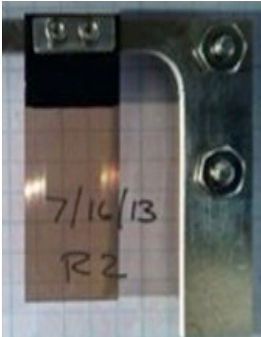
Figure 1.22 - BlueWave Semiconductor nanocrystalline diamond foil post-growth/etch.
