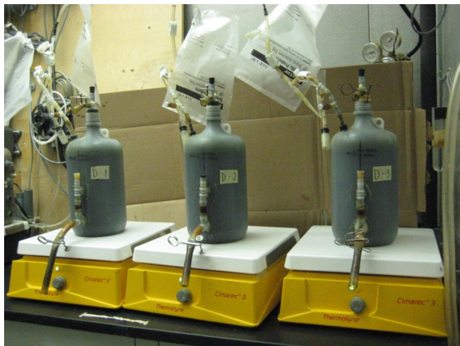
Figure A.2: 3.6L semi-continuous reactor co-digesting chicken litter with dairy manure.
