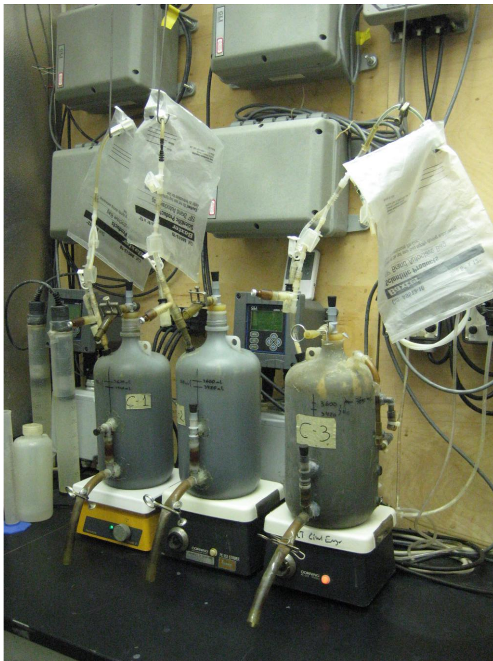
Figure A.1: 3.6L semi-continuous reactor treating dairy manure alone.
