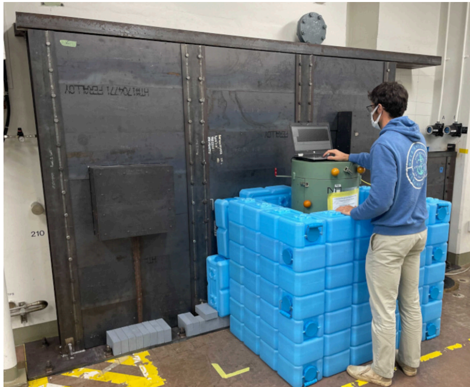
Figure 3.5: Russian doll shielding water bricks. Background shows the lead shield wall.
