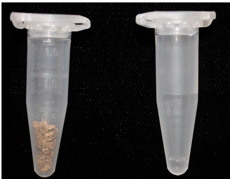
Figure 11. Batches of walnut drill shavings were collected into 1.5 ml safe-lock microcentrifuge tubes (left); solutions of isolated DNA were used for PCR amplification (right).
