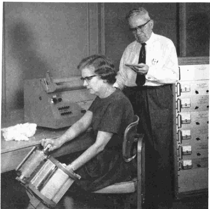
Figure 12. A digital fibrograph for measuring cotton fiber length is shown along with the transistorized control cabinet to the right. Samples are prepared for scanning with the fibrosampler in the left foreground. The digital model fibrograph is readily adaptable to automatic data acquisition.
