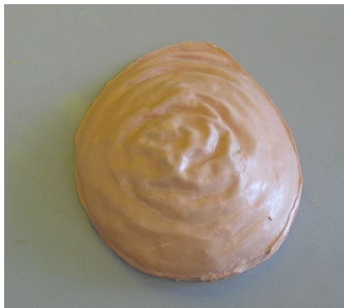
Figure 11: Final breast phantom created using Dragon Skin and silicone gel
