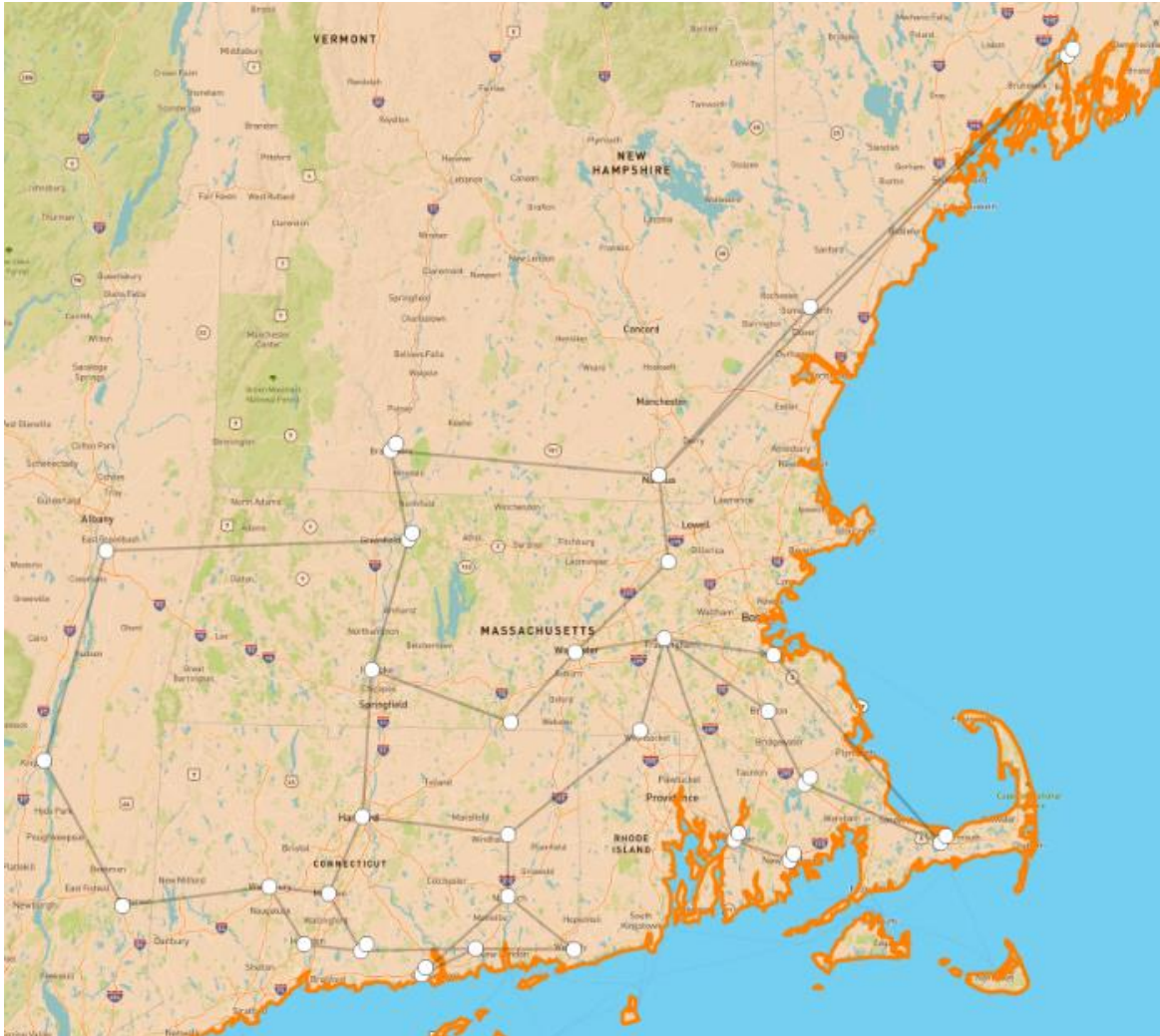
Figure 4.2 One-line diagram of the New England 39-bus system (for illustration only)
