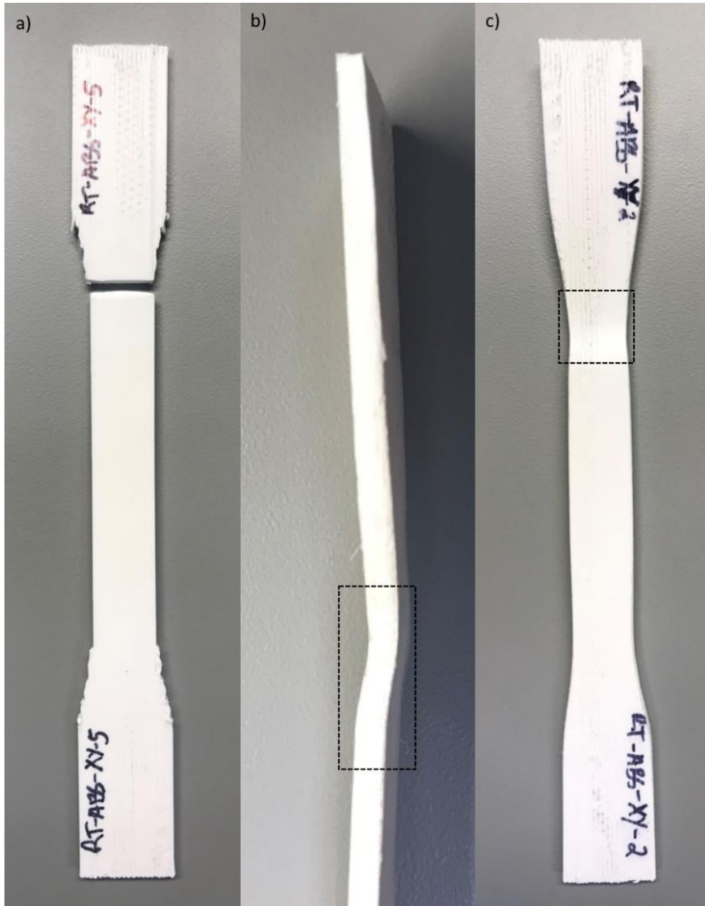
Figure 42 a) typical break of the specimen set. b-c) Demonstrating failure to break but a bow below the fillet region in RT_ABS_XY_2
