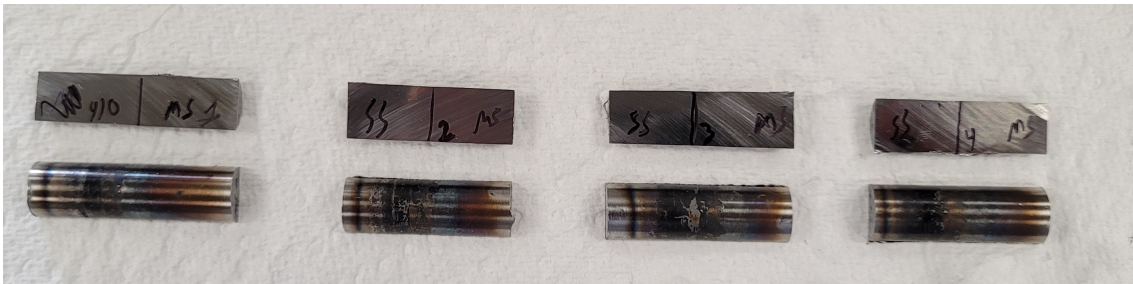
Figure 21: Sectioned gleeble samples after testing
